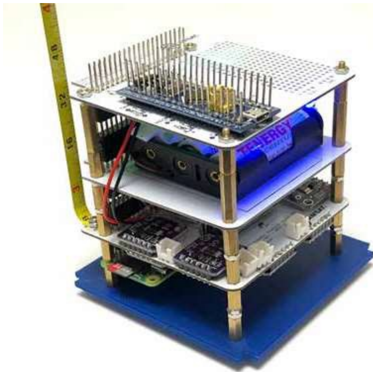
Figure 2- The AMSAT CubeSatSim boardstack: from the bottom, Raspberry Pi Zero WH, Main PCB, Battery Board, STEM Payload Board.
